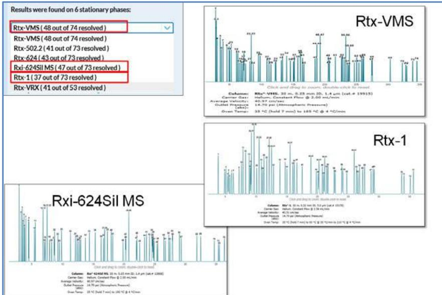
**Figure 2:** Pro EZGC® will show results on multiple phases. The best selectivity will be displayed. This may not be the optimal selectivity for YOUR sample as some components may be present in very large concentrations, masking neighboring peaks.
