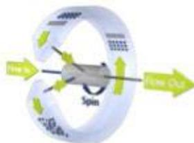
**Figure 1** Separation principle of Centrifugal Field-Flow Fractionation (CF3).
