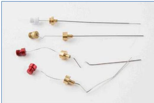
The SPME Arrow was evaluated for 92 VOCs. ISO 17943 only list 63 VOCs. The following results were obtained from 10 mL of water with only a 2 minute headspace extraction @ 60 °C and a 1 minute desorption @ 250 °C.
